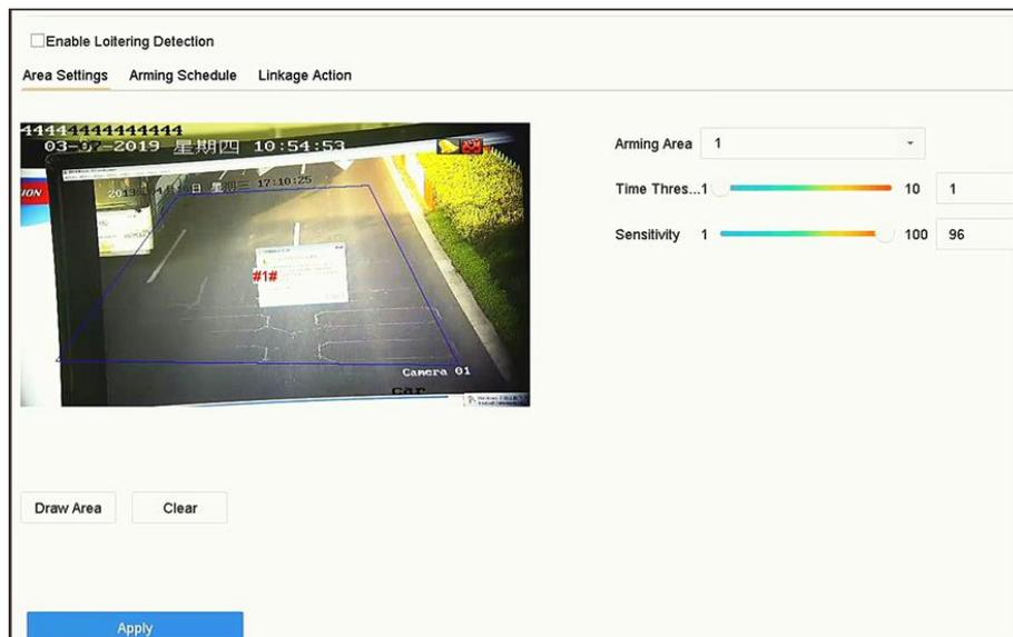
Figure 6-10 Loitering Detection
